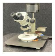
73M is a Manual Die Bond Station which ergonomically positions the cavity atmosphere heated work holder under the Stereo zoom Microscope. The heated work holder is designed to support the operator's hand position as well as multi-stage waffle pack / mirror carousel. The heated work holder and pre-heat station are simultaneously maintained by a touch screen temperature controller,
