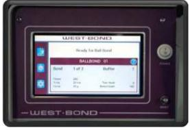
**PROGRAMMING:** The machine may be programmed for up to thirty devices per mode of operation in separate buffers. Each buffer may have up to 21 stitch bonds with individual ultrasonic power, time, force, and loop elevation control data. Program values, action prompts and fault diagnostics are displayed on a 7" LCD Capacitive Touch Screen.
