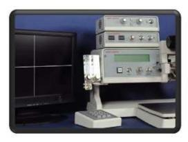
**PROGRAMMING:** Individual loop shape and bond parameters are programmed within specific wire types, where there can be up to 30 wire types per device, each wire type having up to five bonds on a single wire. The three modes of operation, wedge, deep access, and ball share 30 devices.
