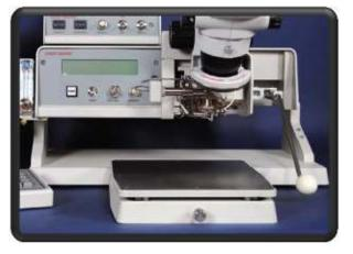
**AUTOMATIC PRECISION** at a fraction of the cost. Microprocessor controlled motors drive both the Y and Z axes for a series of parallel, single or multiple arched wires maintaining identical loop and bond shapes. This system is ideal for bonding high power, high frequency devices where identical bond and loop shapes are critical. In such applications as • Microwave • Semiconductor • RF and • Hybrid products.
