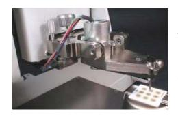
**UNLIMITED DEEP REACH** access to remote bond targets on large packages with WEST-BOND'S new throatless chassis and micromanipulator designs. All machine components, circuitry, and enclosures are arrayed above the horizontal work area, eliminating any restrictions to package size or shape. Manual "E" Series models are available for all microwave, semiconductor, R.F., and hybrid production, and are ideal for repair station or laboratory use.
