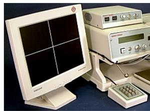
**PROGRAMMING** for different types of wire connections are entered into separate buffers, each with individual ultrasonic power, time, force (high or low) and loop control data. Each type may have up to 100 bonds, and may be repeated for any number of wires for up to a maximum of 6,000 individual bonds. Program values, action prompts and fault diagnostics are exhibited on the easy to read 4 line, 40 character LCD sequentially with machine operation.
